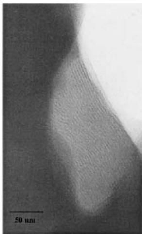
Figure 2 TEM image of aluminosilicate mesostructured material.
